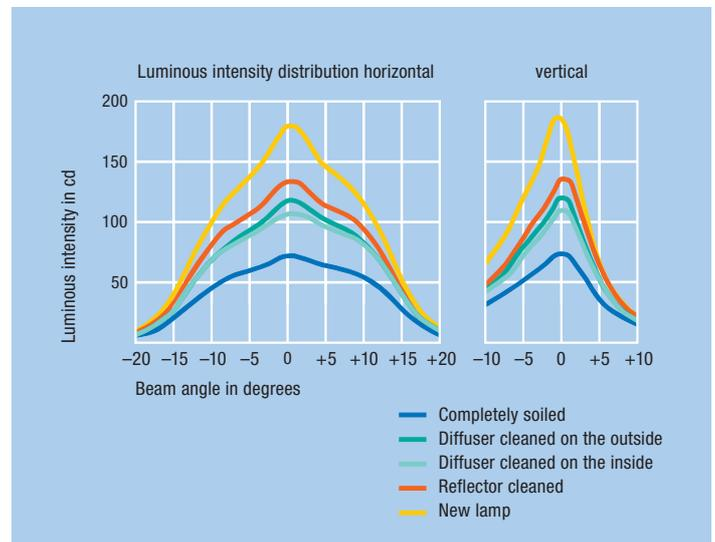
**Effect of soiling and bulb blackening on the signal luminous intensity of a low-voltage lamp**
