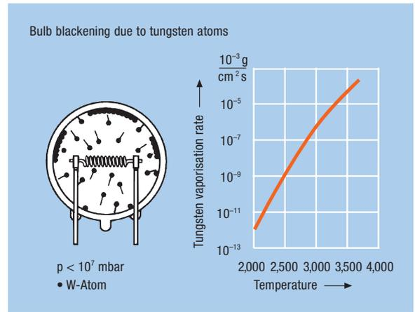
Fig. 1: Vacuum lamps with tungsten vaporisation rate
